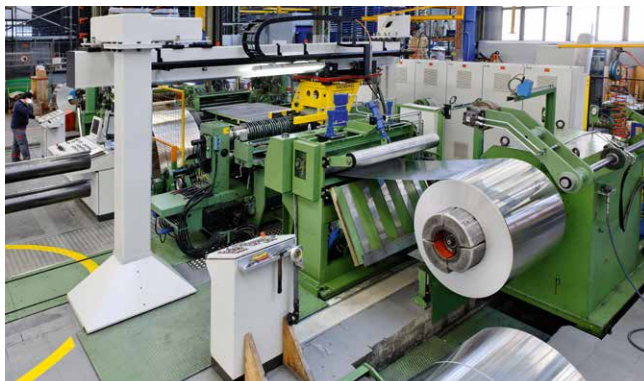
Installation de refendage
